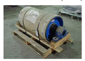
• 18 x 32 Lagged Pulley with Shaft
