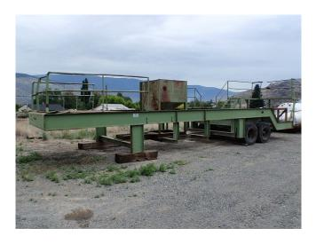
Low Boy Trailer. 10 ft. wide x 40 ft. long. 16 in. x 5 1/2 in. I-beam. Tandem Axle. Light and brake connectors. Walkways and hand rails.
