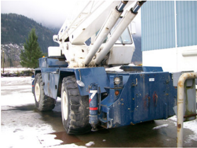
Lorain / Koehring LRT 330 Mobile Crane. 81 FT Boom.
