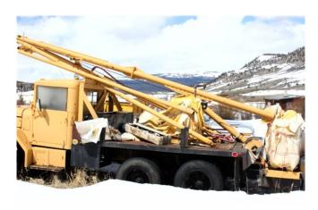
Longyear 34 Drill, Truck Mounted. Driven by 300 Detroit Diesel Engine. Comes With 2,000 Ft. of B-Rod
