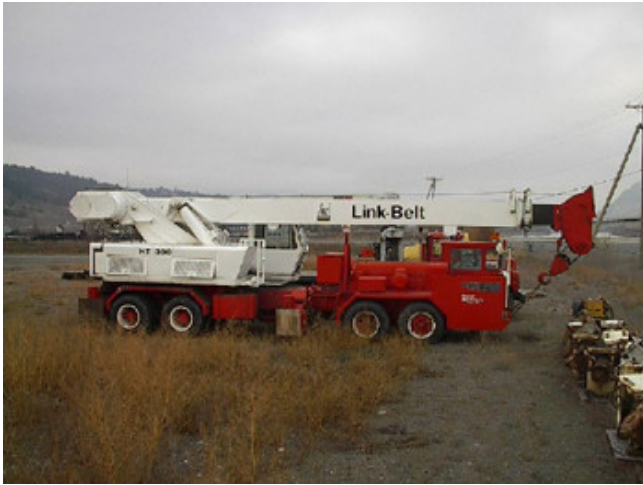
Link-Belt H300. 30 Ton Mobile Crane.
