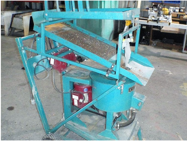
Knelson KC-MD7.5 with KC-VS7.5 Vibrating Screen
