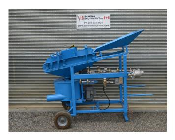
• Designed to recover 94-98% of +325 mesh free placer gold. Precise control of water pressure and flow. Ideal for bulk clean up of .20 inch (5 mm) minus concentrates. Stainless steel bowl with steel wear rings. Site portable.
