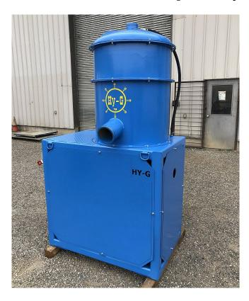
Hy-G HR10 Centrifugal Gravity Concentrator – Hard Rock
