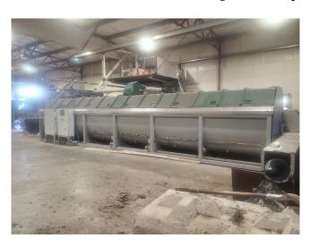
HotRot Turn Key In Vessel Composting System
