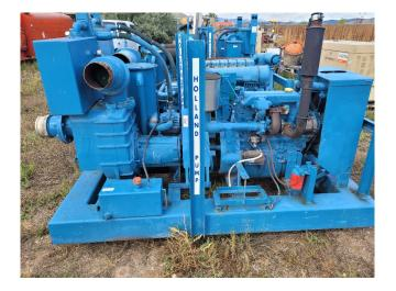
Holland 6in x 6in Self Priming Portable Pump
