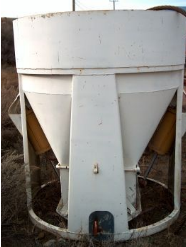
Hoist Type cement bucket. 5.5 yard. Air activated clam shell discharge
