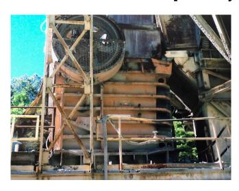
Hewitt Robins 4248 Jaw Crusher Package with Deister 54" x 28' VGF, Discharge Conveyor, and Steel Frame Stands.
