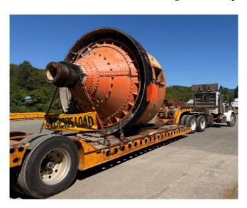
Hardinge 8ft Dia. x 4ft Long Conical Ball Mill
