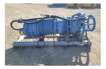
GPM Heavy-Duty Submersible Even Wear Slurry Pump
