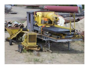
Gold Mining Equipment. Placer/Tailings Pilot Plant. Trommel and Ball Mill, plus Full Size Gold Concentrating Table. All on 35 ft. Highboy Trailer. Complete with feed conveyor and generator
