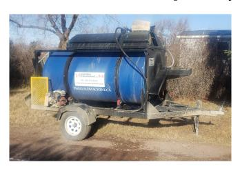
The Model 10 is a small scale and testing plant capable of 10 Cubic Yards Per Hour. The system is run by a 6.5HP Honda gas motor. Water is supplied by the included 2 in. Honda gas pump. Fully contained on it's own trailer ready for transport and can be set up anywhere in under 20 minutes.
