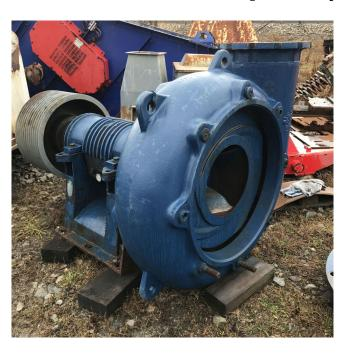
Inlet: 14 inch.Outlet: 12 inch.Impeller: 28 in.
