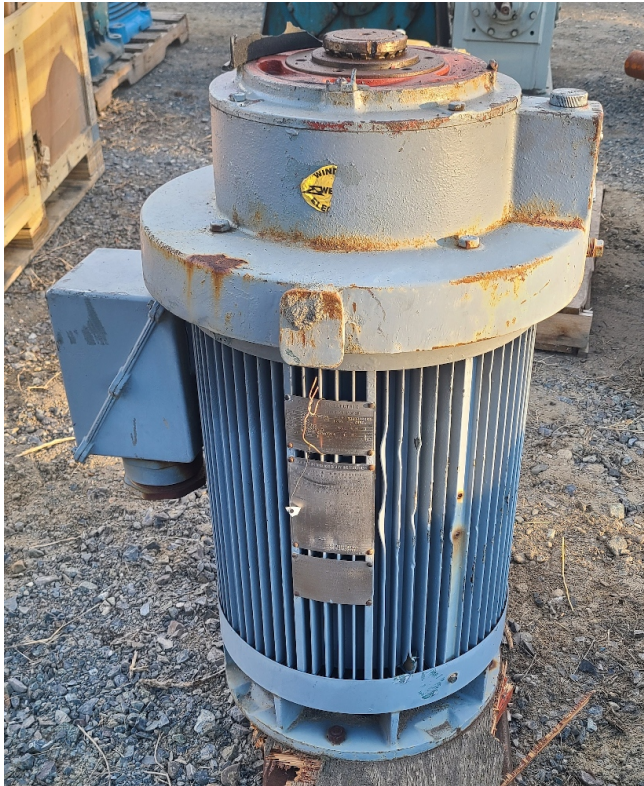
General Electric 75HP Vertical Motor
