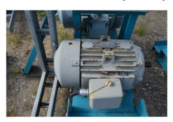
Horsepower: 30Voltage: 575RPM: 3550Frame: 286TS
