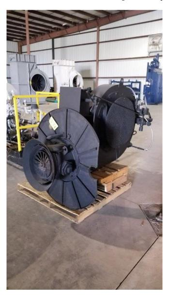
Model: AF-75Combo Oil/GasMotor: 75 HP
