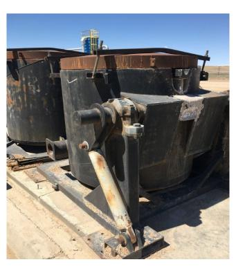
Gas Fired Tilting Furnace Package
