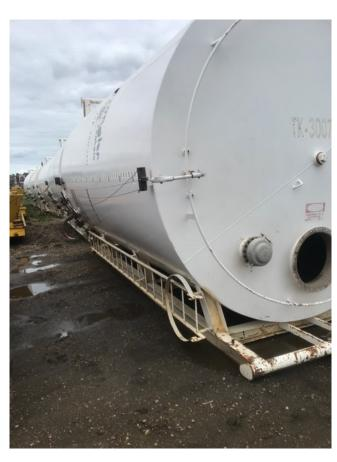
• Capacity: 400 Barrel (16,500 Gallons)
