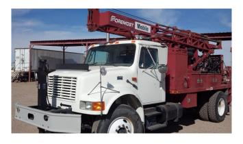
The B-58 can be configured for auger, rotary, diamond coring or percussion drilling.
