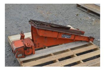
FMC 36" Syntron Vibrating Pan Feeder
