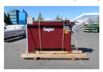
Model: 23-200Horsepower: 5 HPVoltage: 230 Volts
