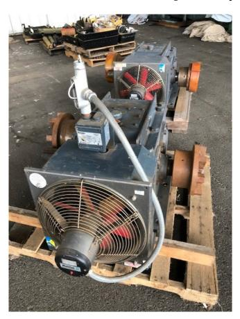
Model: 385A1-CBRation: 2.812Input RPM: 1750Output RPM: 622.3
