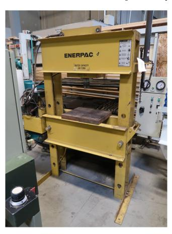
Capacity: 100 TonHorsepower: 1.5 HPVoltage: 115 VoltSingle Phase
