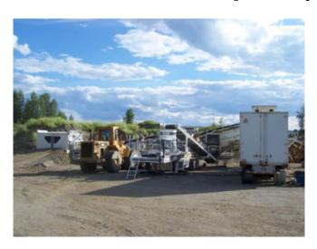
Elruss portable crushing plant. 3800 Hydrocone, 6 x 20 - 3 deck screen, 36 inch stacking conveyor and power van with 365 KW gen-set.
