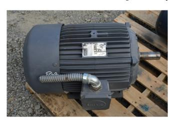
Voltage: 575 VoltHorsepower: 20 HP
