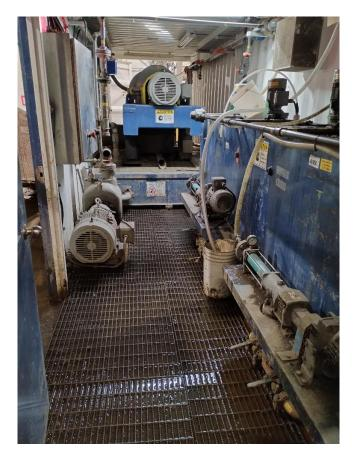
Elgin ClearWave 40<sup>™</sup> Containerized Dewatering System
