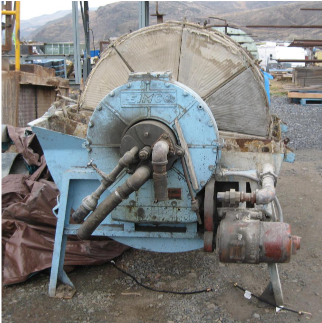
Eimco 4ft Dia. x 4ft Long Disc Filter
