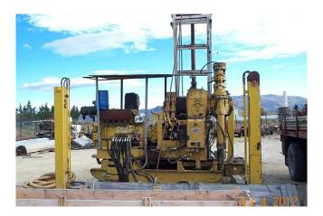
Edeco Stratadrill 80 Diamond Core Drill with HQ Chuck, 6 Cylinder Deutz Drive, Located in New Zealand
