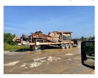
Eagle Ultramax 500 Portable Impact Crusher Plant
