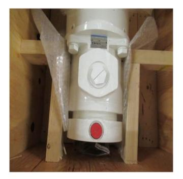
Dynex PF4000 Series Checkball Piston Pump with 15HP 575V Baldor Explosion Proof Motor
