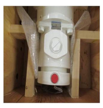
Dynex PF4000 Series Checkball Piston Pump with 15HP 575V Baldor Explosion Proof Motor
