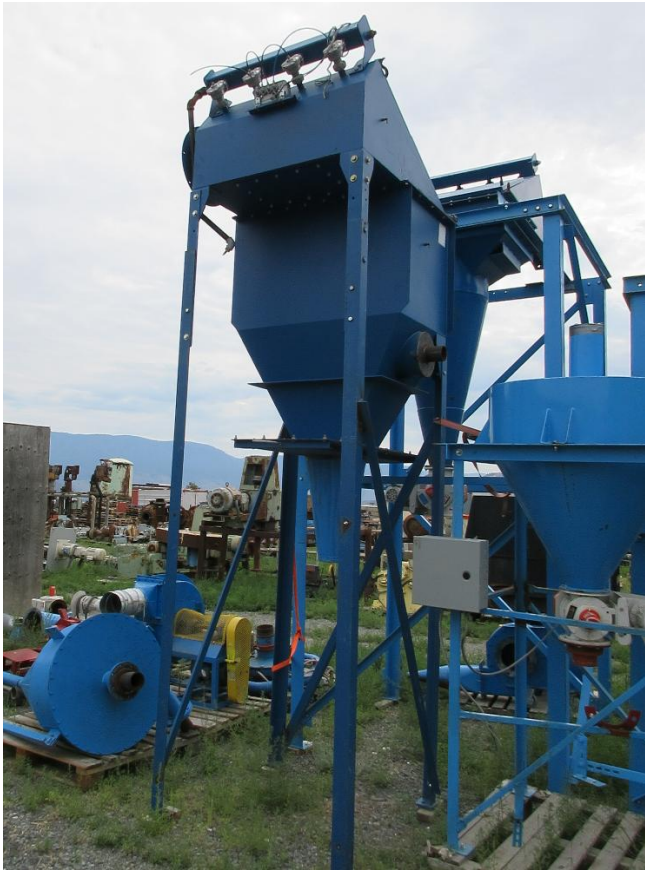
Donaldson Power-Core CPC4 Dust Collector
