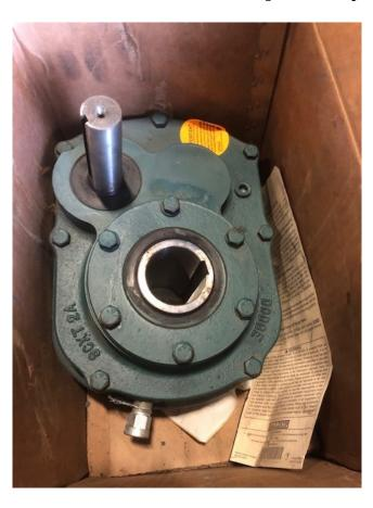
Dodge SCXT225 Shaft Mount Screw Conveyor Reducer
