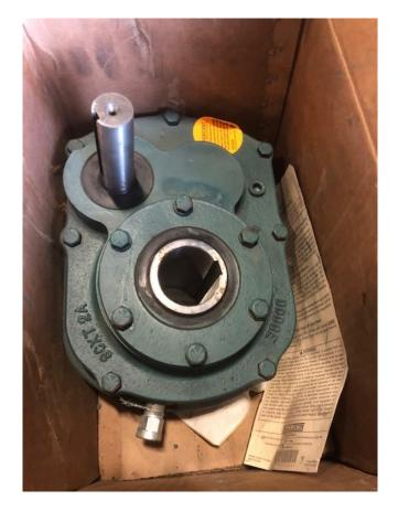
Dodge SCXT225 Shaft Mount Screw Conveyor Reducer
