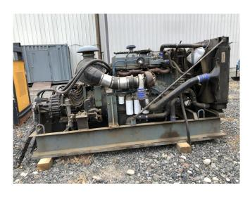
Detroit Diesel Series 60 Engine with Allison HT750 Transmission
