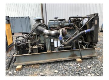
Detroit Diesel Series 60 Engine with Allison HT750 Transmission
