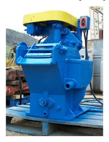
Denver #7 Sub A Lab Flot Cell. Rubber lined cell. Complete With 1/2 HP - 60 Hz. Single Phase Motor.
