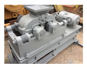
• Driven by Linkbelt <u>3 HP</u> gearmotor.
