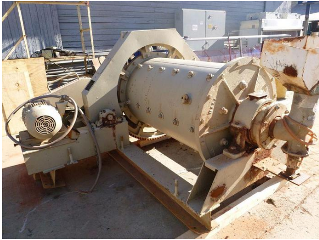
Denver 30in Dia. x 54in Long Ball Mill
