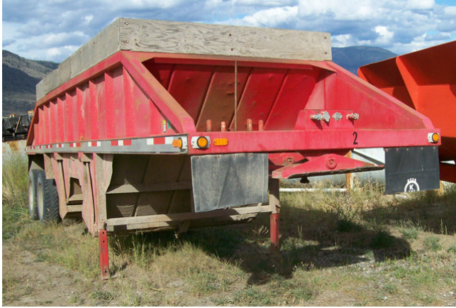
Decap Belly Dump Trailer. 8 Ft.W x 32 Ft.L x 8 Ft.H. Air Operated Clam Gates.
