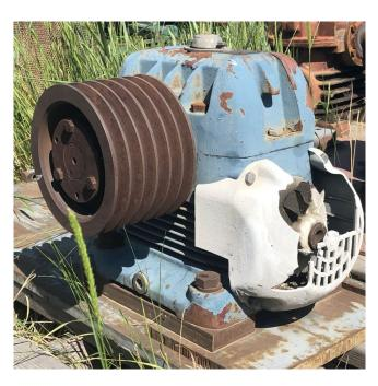
Size: AU400-BRatio: 10:1-RInput shaft: 1.25"Output shaft: 1.75"
