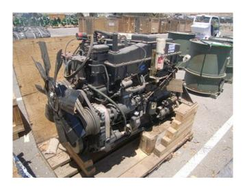
• Cummins Diesel Engine.
