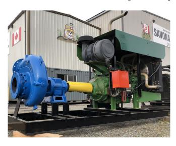
10 inch Cornell Centrifugal Pump Model: 10RB-F18DB
