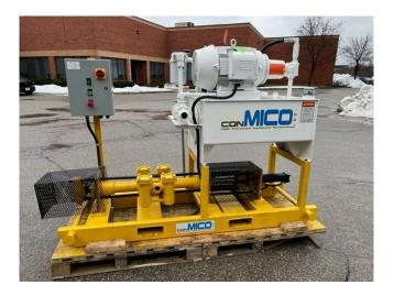
ConMICO Electric/Hydraulic Grout Pump
