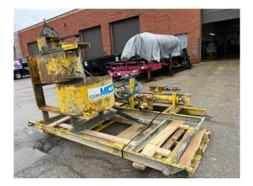
ConMICO Co-Pak PCS-13-400 High Pressure Grout Plant
