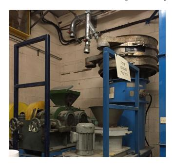
Crushing plant includes Mainland <u>Bucket Elevator</u>, Denver <u>Roll Crusher</u>, Marcy <u>Cone Crusher</u>, Sweco <u>Circular Screen</u>, and Morse Brothers <u>Jaw Crusher</u>
