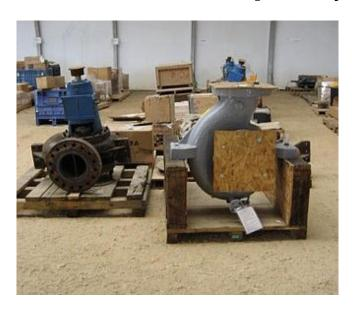
Input: 10 inches.Output: 10 inches.Impeller: 15 in.Mechanical seals.
