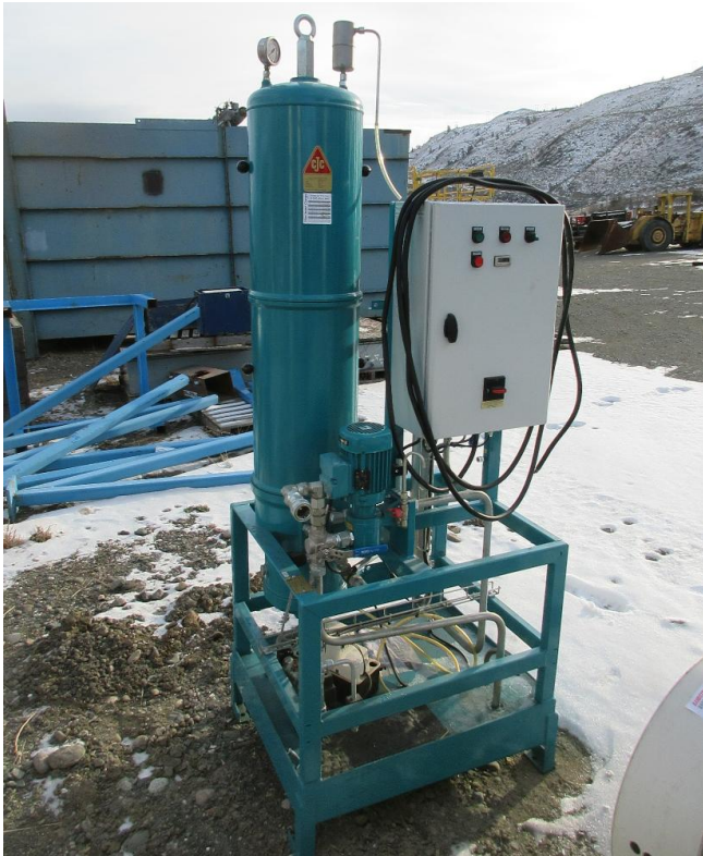
CJC PTU.327/180 Oil Filter Separator
