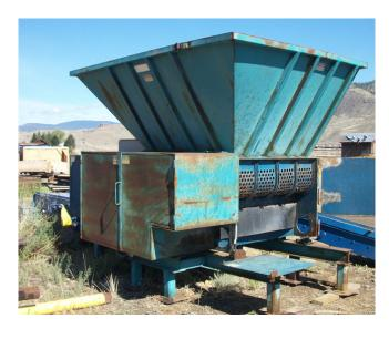
Challenger 400 Pallet Grinder. Driven by 50 HP - 440 Volt Electric Motor. C/W Shaft Mount Reducer and Electrical Control Panel.
